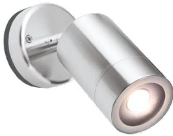
A compact, adjustable, direct or indirect accent used for grazing walls or other accent illumination tasks. The luminaire is constructed from 316 marine-grade stainless steel with ElectroPolishPlus™ surface treatment, to provide long-life, even in coastal environments. This luminaire is ideal for use in modern architectural designs, and features Lumascope's d5 driver technology for advanced dimming and control options.
