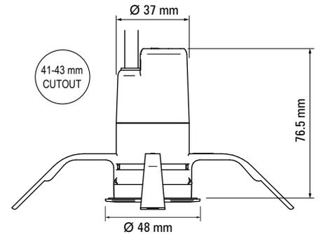
4. Fold legs up on the ceiling clip and insert into hole and feed LS9407LED cable through mounting clip, connect to supply as per instructions supplied with the LS9407LED and test.
