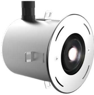
The Nero NE1 is a swimming pool rated luminaire constructed entirely of marine-grade 316 stainless steel. It utilizes a special alignment feature to ensure the beam of light is perpendicular to the installation surface, even if the pre-installation blackout niche is not. The use of LEDs allows for the creative introduction of color and improved energy-efficiency. This luminaire is suitable for saline waters.
