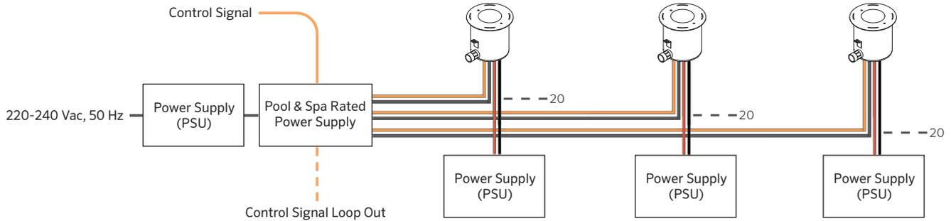
Up to 20 luminaires per run under the following conditions:
