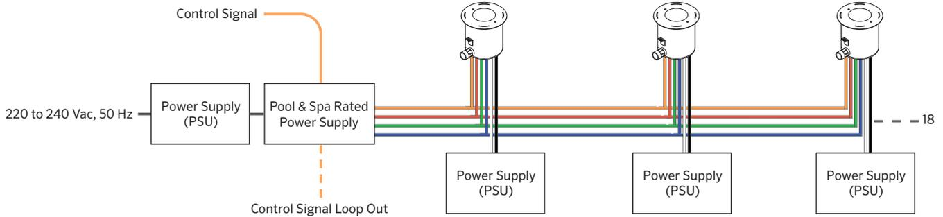
Up to 18 luminaires per run under the following conditions:
